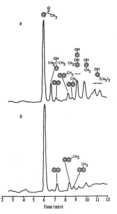
Fig. 1. Gas chromatograms of seawater extracts of bunker fuel. a. Recovered by chloroform extraction. b. Recovered by pentane extraction.
